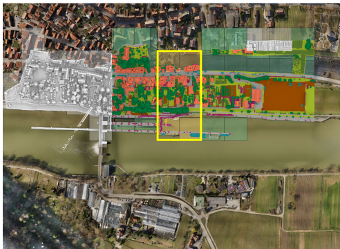
Figure 2: Partition of the H3D(PC) dataset (epoch March 2018) into training (colored by class colors), validation (colored by class colors and marked by yellow box) and test set (grey).
