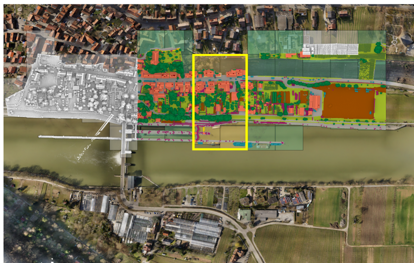
Figure 4 – Partition of the H3D(PC) dataset (epoch March 2018) into training (colored by class colors), validation (colored by class colors and marked by yellow box) and test set (grey).
